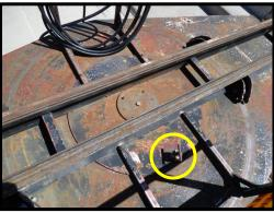
Spring loaded keeper pin, holds table in position, pull pin to turn table. Load MUST be balanced to the center of the table.
