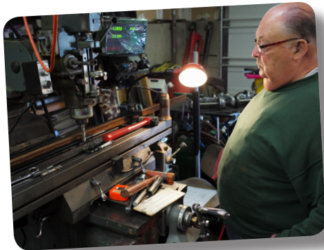
Nick Buell milling steel rail to upgrade a switch for the new wye
