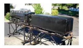
Pacific 4-6-2 Locomotive complete and running with prints. Passed all tests for 10 years. Steel boiler and tubes.
